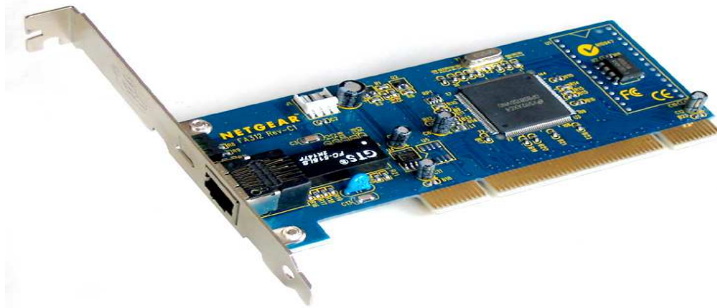
Fig 2 NIC Card Hardware structure
